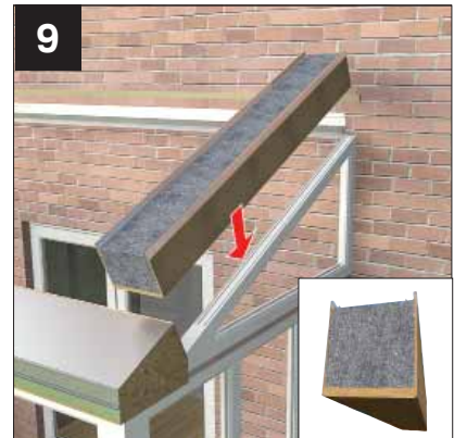
Locate end panel (s) onto the rear wall plate shelf and box beam shelf. Ensure OSB boarding on end of gable panels are flush with the end of the beam. Note: if there is glazing against a return wall see page 25. Marked with a yellow label, all gable end panels are supplied with OSB (timber panels) to the inside face. DO NOT SNIP RETAINING STRAPS.
