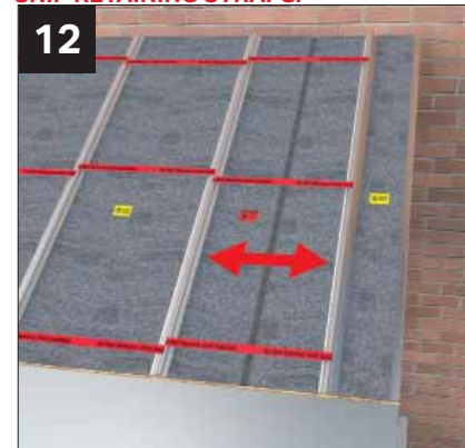
The red labelled panels are always installed last. DO NOT SNIP RETAINING STRAPS.
