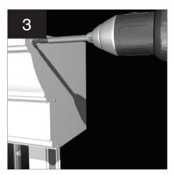
Secure the end plate (CRN003) into position using the fixings provided (CRN008).
