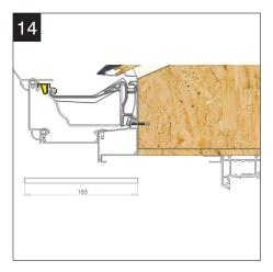
**EXTENDED SOFFIT ONLY**: In an extended soffit situation, cut the soffit board 185mm in width in order to fit into the soffit channel and support section.
