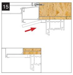
To fit the soffit board, angle the board fully into the soffit channel, once in the soffit channel pull back to slot into the support section.
