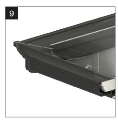
Fit remaining cornice components and secure using two tie wires. Fix wires into the barge board face below the top line of the cornice (tie wires may require bending to suit). Fix using self drilling screws CRN010.
