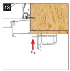
Fix the PVCu soffit channel into the box beam up against the head of the window frame.
