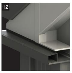
Cover the corner joints by modifying the PVCu fascia corner supplied and fit cover shelf as shown. Support shelf at frames using timber or similar
