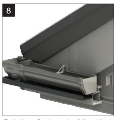
Fit the lower Cornice section followed by the guttering. Use face-fix gutter bracket supplied to secure gutter at mid-span of returning gutter as shown.
