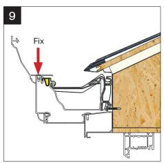
Temporarily support and fit the upper cornice section, using the fixings provided (CRN007). Secure the corners using the cleat (CRN001) and fixings (CRN006) as shown in step 4.
