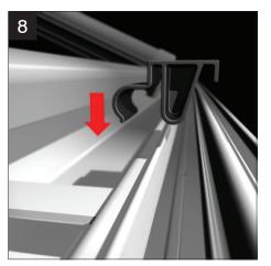
Once lower and middle sections have been fixed and secured, clip fit the support brackets (CRN002), adjacent to every gutter bracket.
