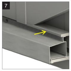
Create and fit cover shelf from 9mm multiboard (not supplied) and point all open joints to weather.
