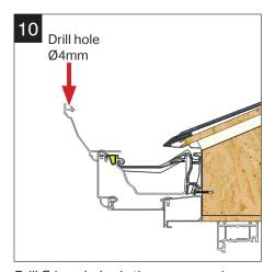
Drill Ø4mm holes in the upper cornice section in line with each gutter bracket.
