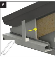
Fit eaves fascia cover and scribe fascia corner before securing in place as shown. For pitches above 26° in pitch - a 90° fascia corner cover will be supplied and should be cut as shown and placed to cover the joint between the eaves fascia and barge board.
