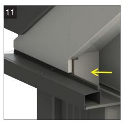
**Extended Soffit Detail** – When an extended soffit is used, a larger void is created between the cornice support and the frames. Scribe a piece of multi-board as shown to cover the internal beam face.
