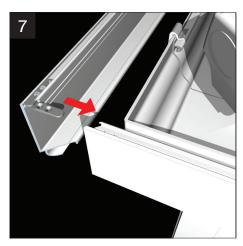
Fit cleats as shown in step 4. Offer up the next middle cornice section. Continue to support lower section as shown in step 6.
