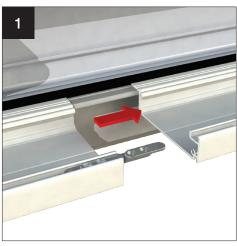
1. Attach the cleat CRN001 using 2  $\times$  CRN006 provided, on each side of the joint. Repeat for each of the Cornice 'layers'.
