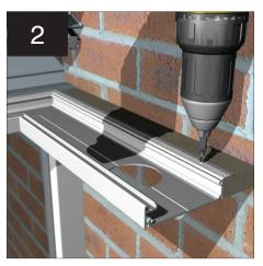
Secure lower section using fixings provided (CRN007).
