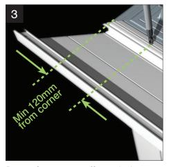
Prior to fitting gutter offer up the lower cornice section then secure into support section using the fixings provided (CRN007). Please note: Always start with the front facet!
