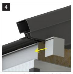
Cut down and slit the supplied NRFCS090 fascia corner trim and fit at beam corner to protect exposed OSB face. (Shown fitted inset)
