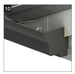
Finally, secure the standard end plate into position using the fixings provided, CRN008. Dependent on pitch, the end plate may require trimming to suit.
