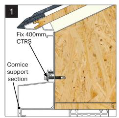
Fix the cornice support section flush to the box beam using RRR025 5.5 x 32mm Hex head drill screws, ensure the fixings are spaced 400mm centers, minimum 200mm from the corners.
