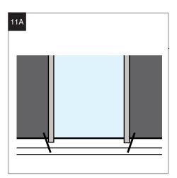
When roof contains a glazed panel, it is recommended to fix either side of the glazing panel into the roof.
