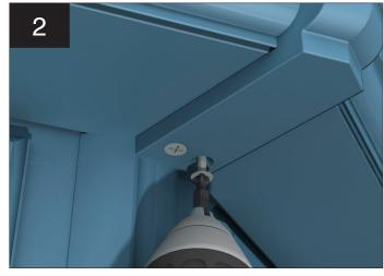
Whilst ensuring that the corner remains located in position, screw fix using self drilling screws CRN007.
