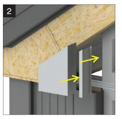
Note: For roof pitches of 26° and above, a firring block and H section frame coupling are provided to create a gable frame infill as shown – these will need to be cut to suit on site. For pitches of below 26° see main guide.
