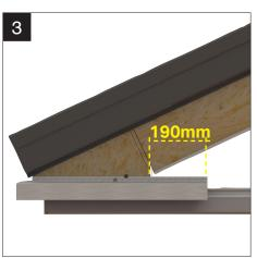
Fix the cornice support section to the end of the box beam at the gable end. The section should extend 190mm past the inside edge of the box beam. Fix with 2 equally spaced RRR025  $5.5 \times 32$ mm Hex head drill screws. Pack as required to square profile around corner (90°).
