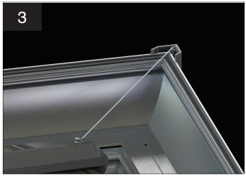
Finally secure the corner by screw fixing the wire tie to the hip cap using self drilling screw CRN010.
