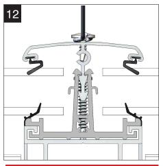
USE CHAA006 (M4 X 13MM SELF DRILL SCREW) TO FIX THE TIE WIRE TO THE GLAZING BAR. FIX THROUGH THE CENTER OF THE GLAZING BAR (±2MM) TO AVOID DAMAGING THE GLAZED PANNELS.
