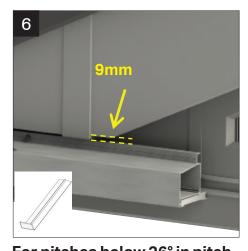
For pitches below 26° in pitch—a 180° fascia cover will be supplied to cover the joint. Fit barge board, leaving a 9mm gap where shown to allow for installation of cover shelf shown in next step.
