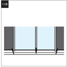
When roof contains 2 or more glazed panels, it is required to fix through the center of the glazing bar.
