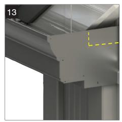
Finally, secure the extended end plate into position using the fixings provided, CRN008. Dependent on pitch, the end plate may require trimming to suit.
