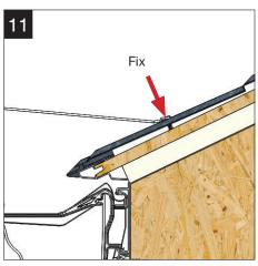
Secure the upper cornice section using the wire ties at each drilled hole. Hook the wire tie into the hole in the upper cornice section and screw fix into the roof using CRN010. Ensure the upper section remains parallel to the frames/roof line.
