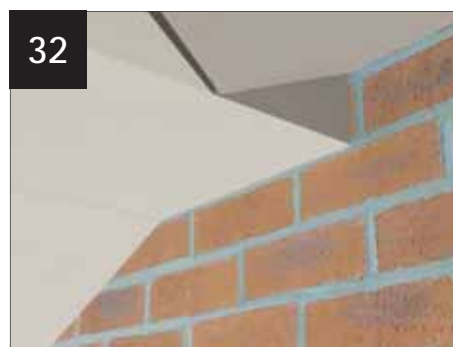
Now fit the plasterboard – the detail where the valley abuts the host wall should look as shown.
