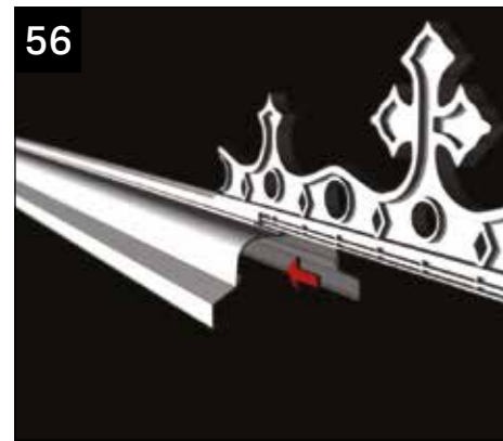
Slide the creasting into the ridge channel. The last section of creasting (by the house wall) may require cutting to length. Some creasting options clip over the ridge body.
