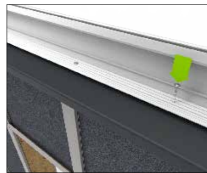
Lower the eaves into position on the cill. Secure the eaves beam down through the cill and into the top tray using appropriate fixings (NOT SUPPLIED) at 450mm centres and within 200mm of the eaves beam ends. Once secured, fixing heads are to be sealed with an appropriate sealant.
