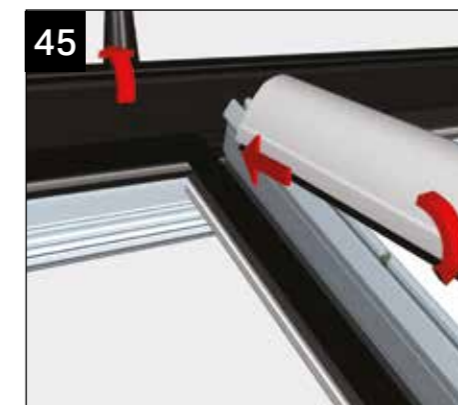
45 Work your way around the roof. The top cap must be lifted into its final resting place (at the ridge) prior to being knocked down over the Anchor clip.
