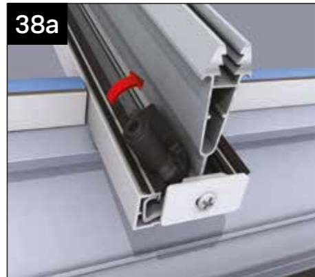
38a Snap off appropriate handed clip (left hand illustrated). Handing marked on base of clip. Line up the rounded edge on base plate next to central web of glazing bar then tuck neatly under gasket side of bar. Rotate clip into position. Push the grommet over the post as shown.
