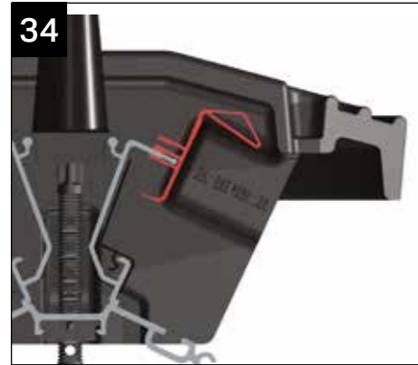
The rain baffle should nestle neatly to form a continuous weather tight joint.
