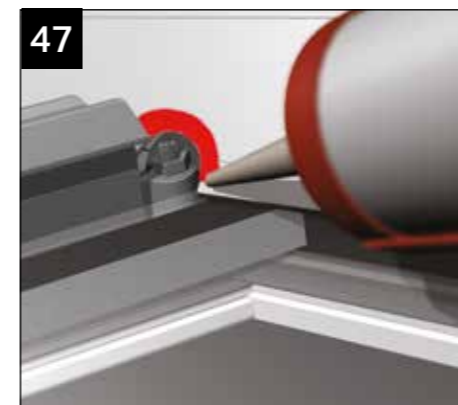
47 Seal around the notched Georgian top cap ready to receive the jack rafter capping.
