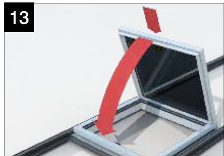
13 When the sealant on the mainframe has cured, re-fit the outer sash by holding vertically and re-engage on to the hinge, before lowering into position.
