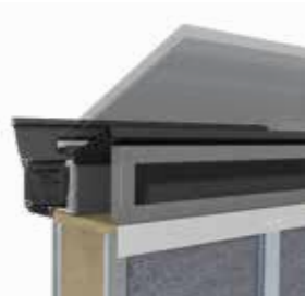
A top tray runs along the top of the hup! walls underneath the eaves beam. The clips are secured into place by fixing through the top tray. Raked frames must be used on lean-to roofs as the walls cannot be raked and meet a glass panel/starter bar. Internally the top tray meets the edge of the internal pelmet or it can be wider.
