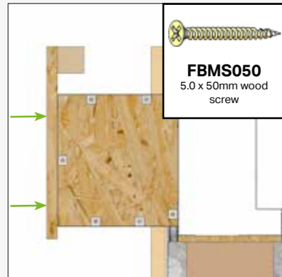
Fit the OSB fascia to the fins in line with the top of the battens using 6x FBMS050 per fin.
