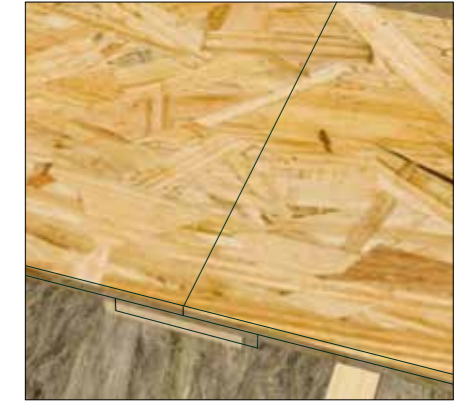
You may encounter panel joints that cannot be supported by either the tongue and groove connection or by a 2x2 firing. In this instance, 6x1 timber is provided to support these joints. Cut the timber to the length required, glue one side and position underneath joint. Lay next OSB in position and nail through to secure.
