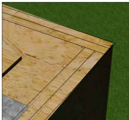
The corner overlap on the opposite side will end slightly different to the first corner. The front elevation OSB fascia will finish flush with the end of the beam and the side OSB fascia will sit flush with the external face of the front OSB fascia.
