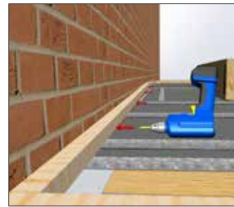
Securing batten to host wall
