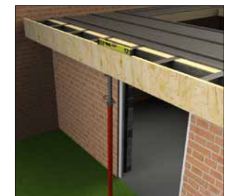
Use a prop to level up the joint before the final fixings.
