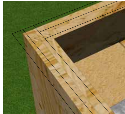
Panel 2a should sit past the external face of beam 1 (in this example) and finish flush with the outside face of OSB fascia 1a as above.
