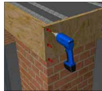
OSB fascia panel joint at corner
