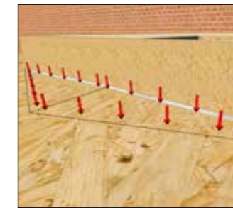
Cricket to L shaped alum section and deck
