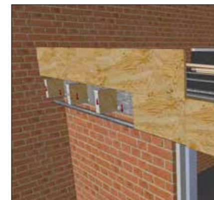
Place fascia panel 1b into place overlapping panel 1a.
