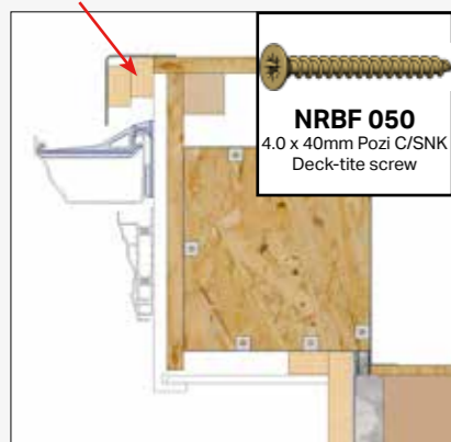
Fit the gutter, heritage fascia (including covers) and drip detail (cut deck to suit your drip detail) as per Classic - Standard and Extended Soffit section (pages 46-48).
