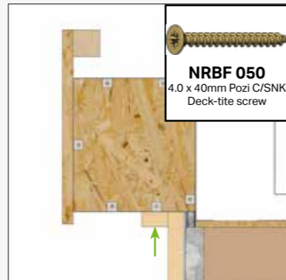
Fix the 2x1 batten to the underside of the fins using 1x NRBF050 fixing per fin.
