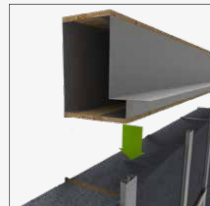
Place the box beam onto hup! walling and align against the inner clips.
