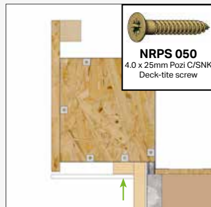
Fit the vented soffit board into place and fix through into the 2x1 batten using 2x NRPS050 fixings per length at 500mm max centres. Use the H section at any corners.
