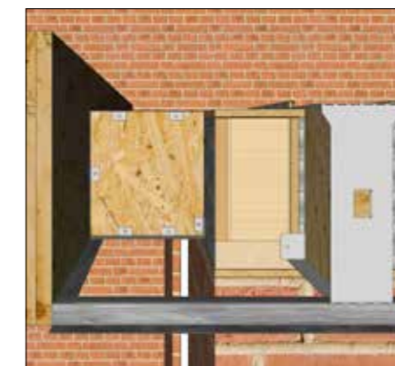
1a onto the Z section, start at the front left hand corner and align the end of the fascia to the end.
