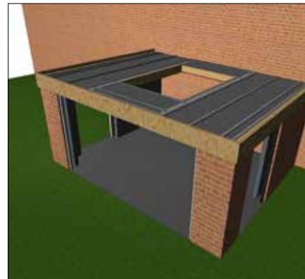
Continue placing and fixing OSB fascia as above across the front elevation and on the return.
