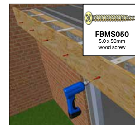
Fix through panel into fin temporarily using FBMS050 fixings.
