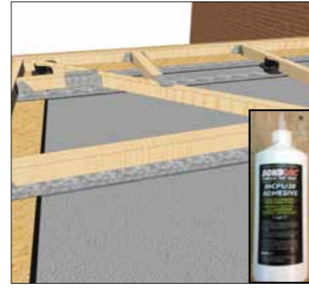
Before placing the OSB deck, use the glue provided to place a line on the timber firings that the deck will lay on. Also glue any joints in the OSB as you proceed around the roof.
