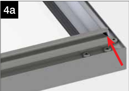
On the hinge side of the sash fill the hole shown above at either end with a blob of silicone.
