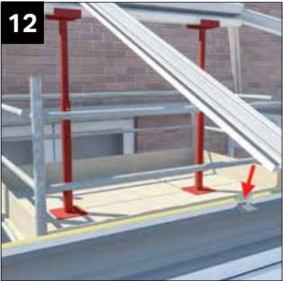
Depending upon the lantern size and options requested, fit hub end transom bar and / or side transom bars. If specified on the job, remove nuts from bolts in transom position and fit transom bar over bolts. Re fit nuts and hand tighten. Check that ridge is level and fully tighten nuts on all bars.
