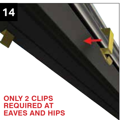
Attach the spring clips (LAN014) to side of the glazing bars. TRANSOM - 2 clips 50mm from the top of the bar. 2 clips 100mm from the eaves. HIP - 2 clips 100mm from the eaves.* top of bar locates on ridge end (see step 16). Push the leg in under the gasket and spring around the underside as shown. Ensure the clips are fully pushed on.
