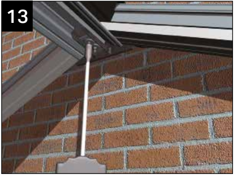
Ensure that the fixing on the eaves moulding and the nuts on the 'crocodile hanger' are tightened up. Also ensure the bolts at the top of the starter bar, are tightened up.
