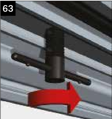
Twist through 90° to locate the T bolt into the ridge capping.
