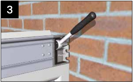
Where the eaves beam sits against the host masonry wall, it has a structural moulding attached to the eaves beam. This has three fixing positions cast into it to allow attachment into masonry – choose the hole that directly lines up with solid masonry and drill a 10mm hole into the host wall. Attach the structural moulding using the M8x80mm anchor supplied. Silicone seal the gap where the moulding attaches to the eaves beam.
