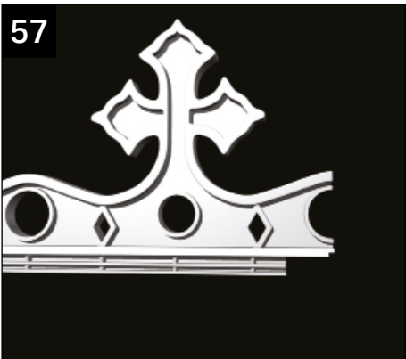
Cut back the underside of the last section of cresting by 40mm.
