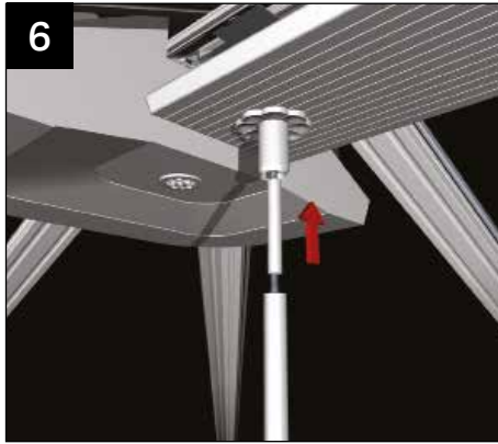
Now cut the PVCu conduit to length, taking care to make allowances for its inset into both the bracket and boss. Take the piece of vertical pvc conduit and slide over the threaded bar and push it home into the ridge cover.
