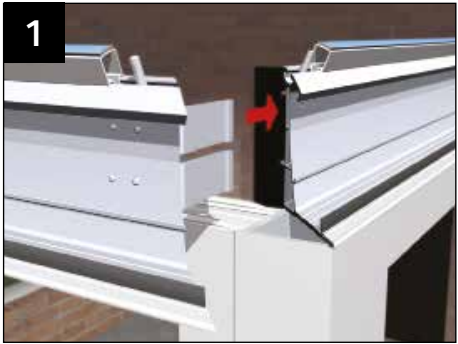
Each eaves corner (90°, 135° and 150°) is supplied pre-fitted with two standard cleats (Georgian 90° illustrated).
