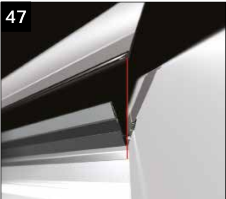
Ensure the jack rafter top capping is lined up correctly (as above) before knocking the top cappings into position. It is not possible to 'tap up' the jack rafter top caps into final position when fitted with anchor clips.
