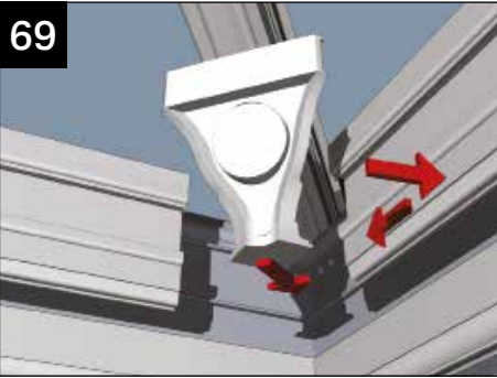
Slot each section of internal fascia into the corner jointer and tap the fascia onto the barbs of the eaves beam. Fit Ultraselect strips into the slots in the fascia
