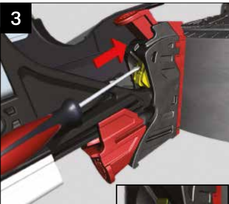
Insert the 5mm wide flat blade screwdriver and gently push against the upper edge of the roller cam (marked yellow).
