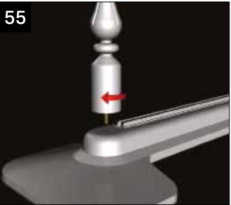
Now down on the ground take the ridge top cap assembly and screw the finial into the radius end capping.
